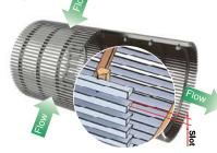
OZ - Circumferential Slot, flow of material on the outside of cylinder (radial)
